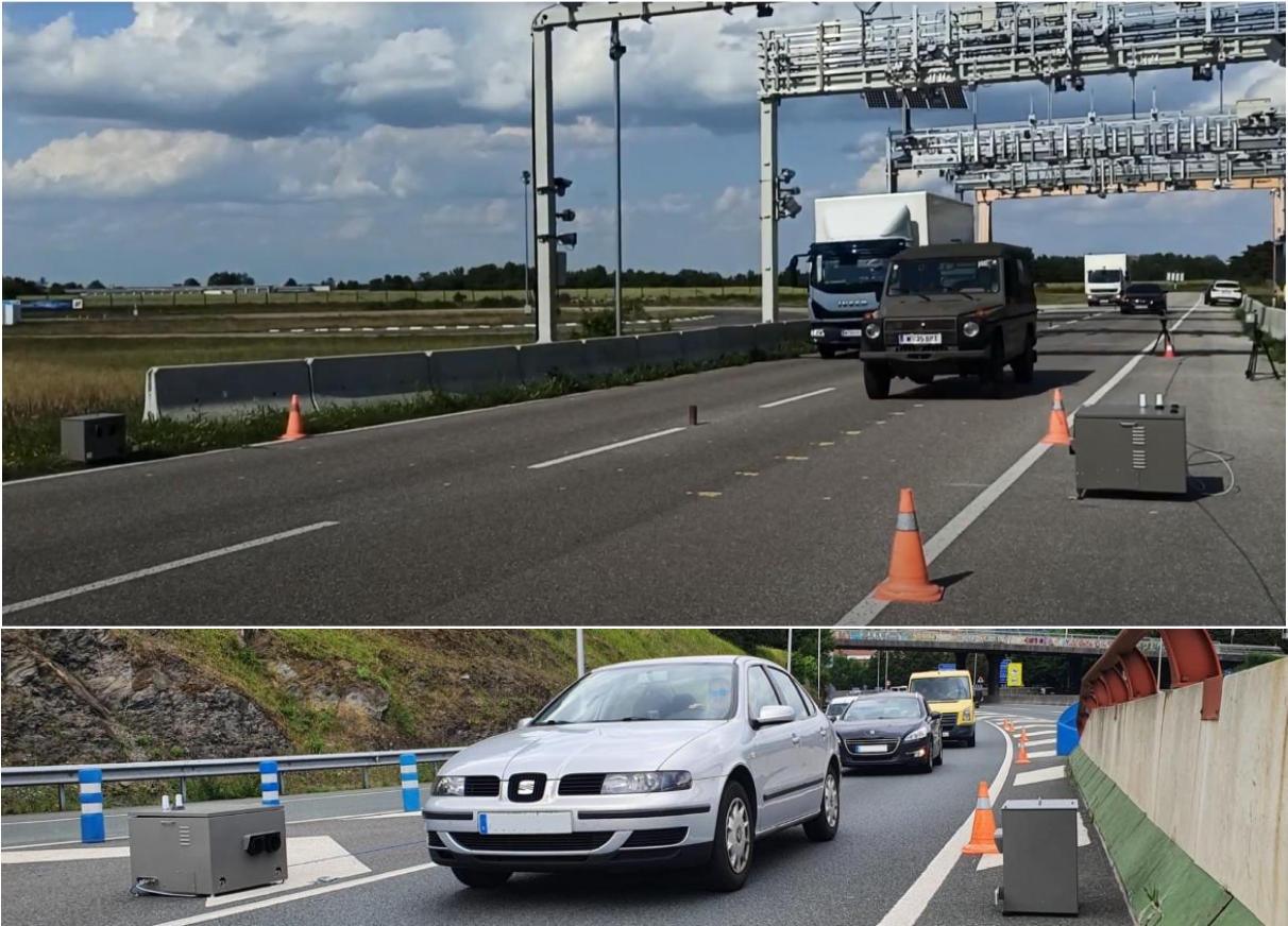
Figure 3: Testing of the measurement system consisting of the measuring station and the reflector on the KTC test track in Teesdorf with different vehicle classes (top); real-world test of the emission measurement system in Spain (bottom) [1], [2], [3].
